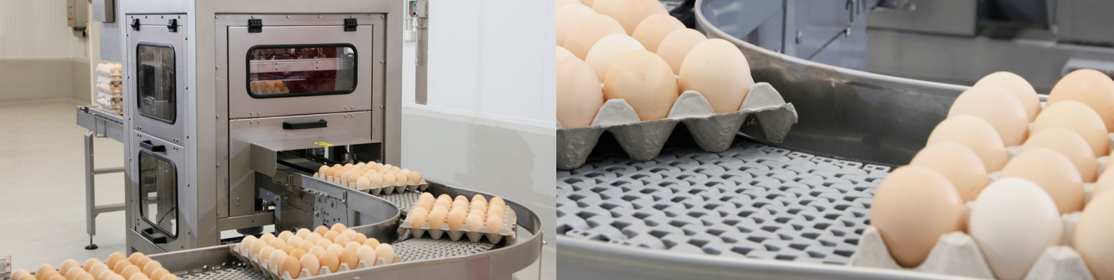
Automatic destacking of transport trays
